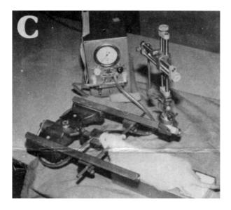
**Figure 2.** Showing the rat fixed in the ear bars, with the tooth plate and ventilation chamber in the retracted position (A); with the upper incisors in position (B); and with the ventilation chamber fixed over the snout (C).
