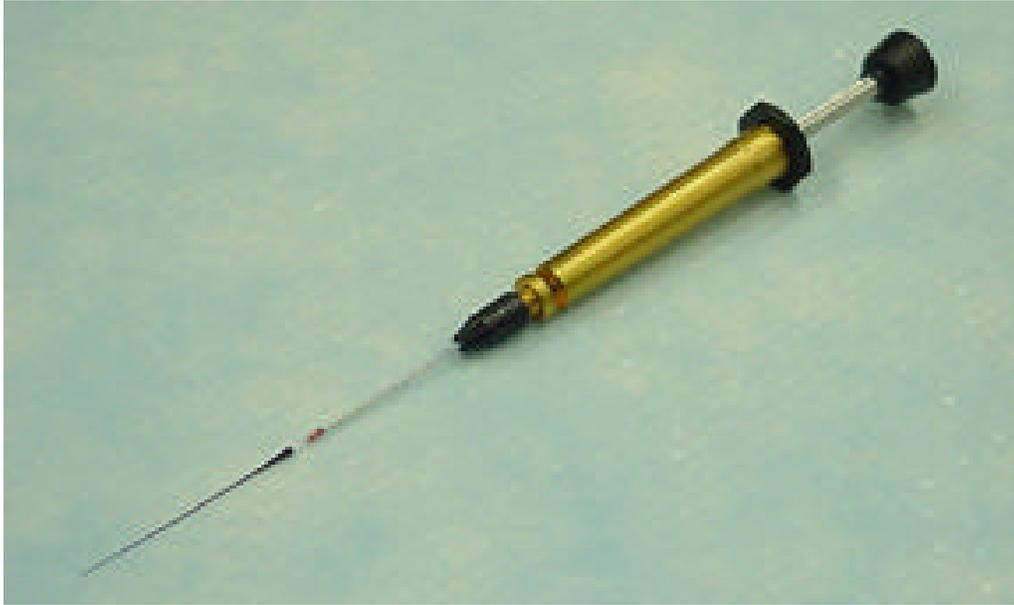
**Figure 4.** Image of the positive displacement syringe with attached beveled micropipette. The micropipette is filled with methylene blue, which was used as a marker to locate the original injection site.
