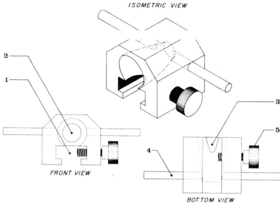
**Figure 1.** Schematic illustration of the ventilation adaptor in front, bottom, and isometric views. 1. Channel fitting over tooth plate. 2. Ventilation chamber. 3. Upper incisor notch. 4. Brass tubes to respirator. 5. Manual set screw.
